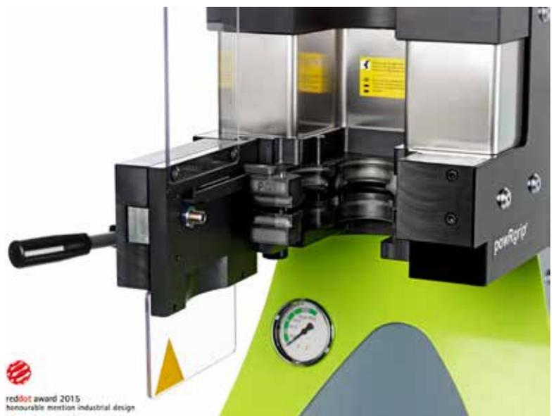
The easily exchangeable clamping inserts of the automatic clamping unit PGU 9500 allow the clamping of tools with shank diameters ranging from 0.2 to 25 mm, without prior parameter setting.
